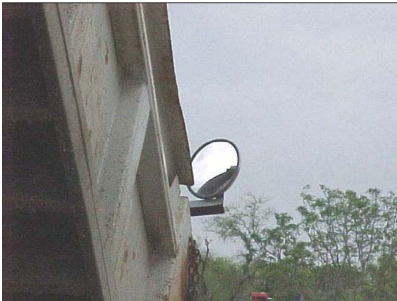
Figure 4-34-C. Mirror to View Rock in Truck and Rock Flow.
