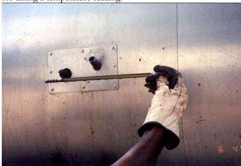
Figure 4-5. Thermometer Removed from Distributor Tank.
