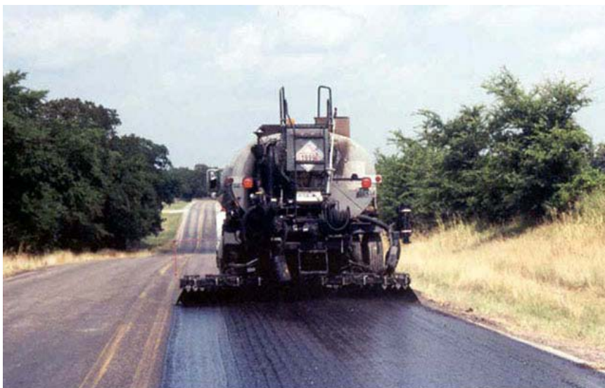
Figure 4-3. Typical Asphalt Distributor.
