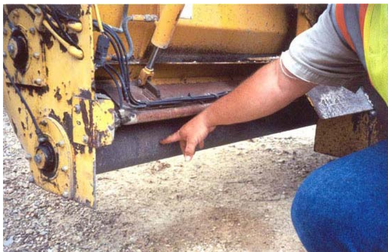
Figure 4-33. Discharge Roller on Aggregate Spreader.
