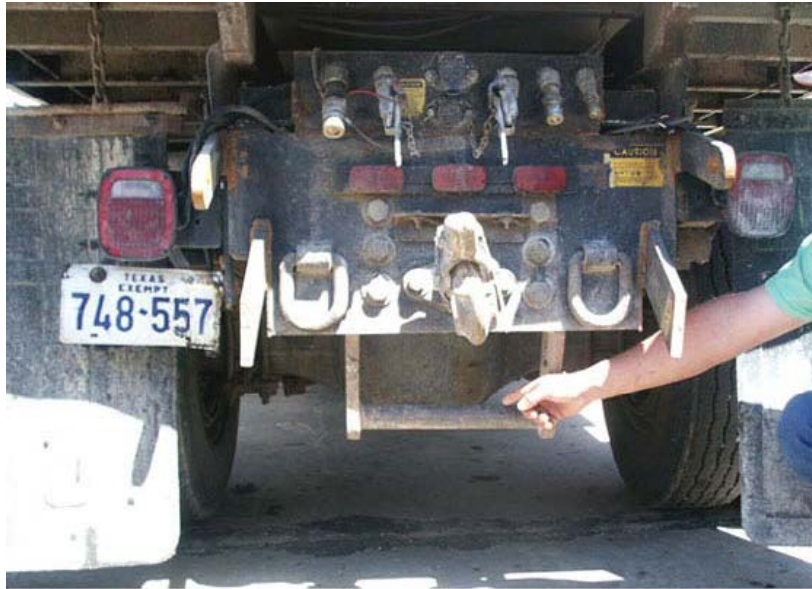
Figure 4-38. Truck Hitch to Connect to Aggregate Spreader.
