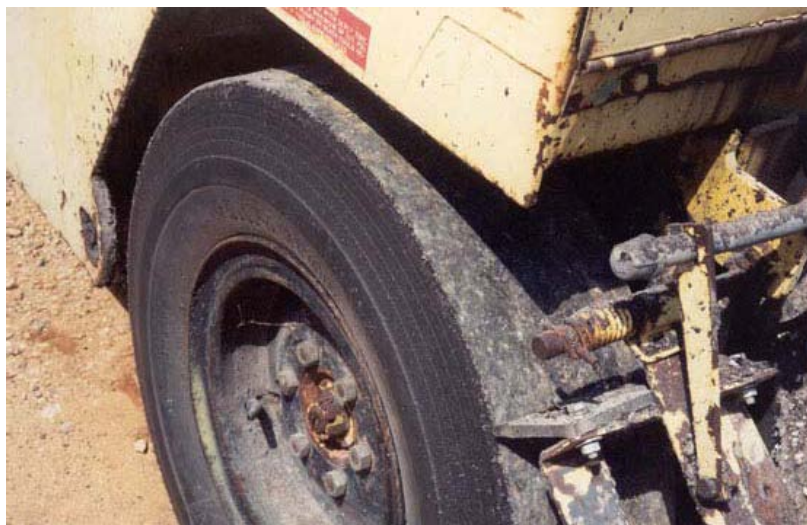
Figure 4-41. Smooth-Surfaced Pneumatic Tire.
