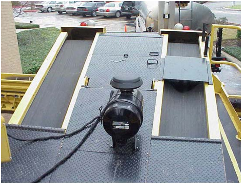
Figure 4-30. Belt Conveyors on Aggregate Spreader.
