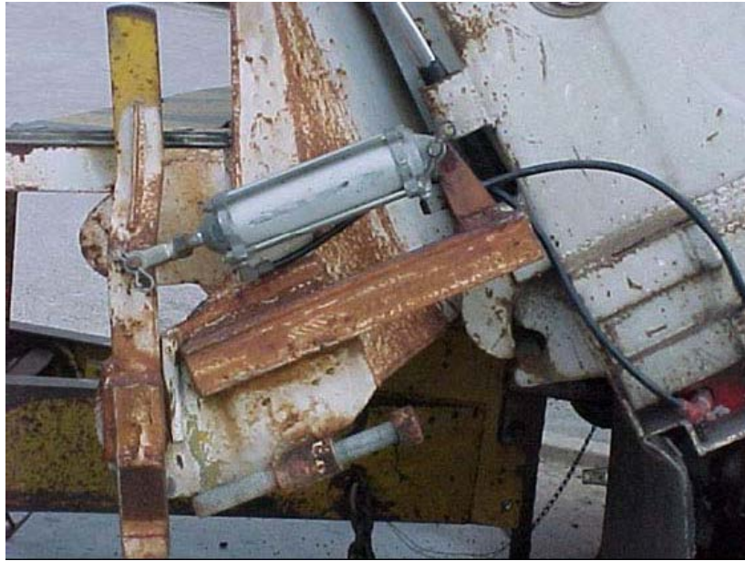
Figure 4-34-D. Air Cylinder to Open/Close Spreader.
