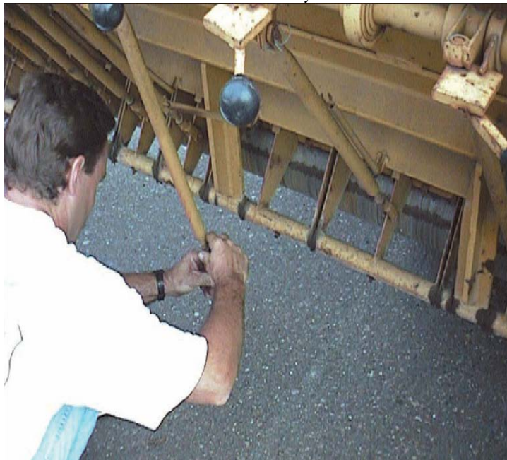
Figure 4-35. Chip Spreader Calibration.
