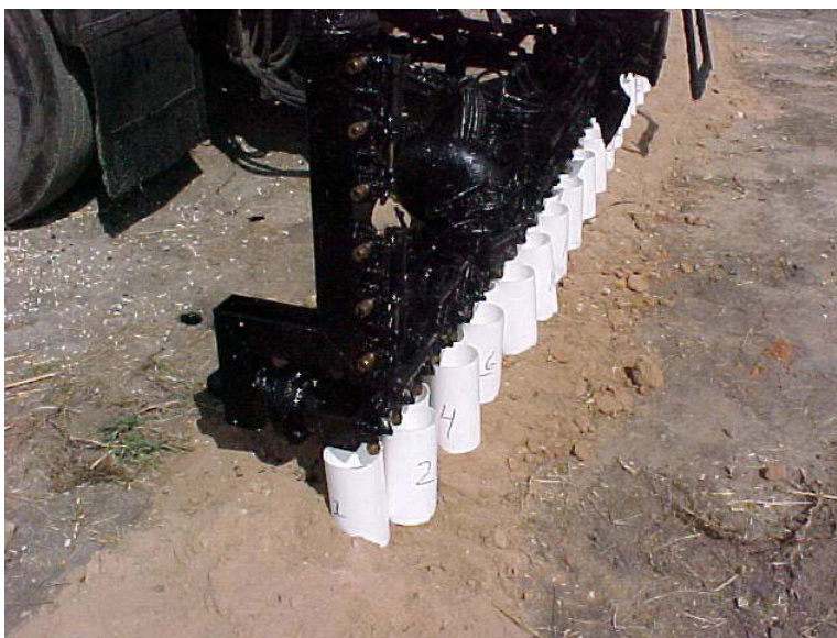
Figure 4-21. Calibration of Asphalt Distributor Spray Bar.
