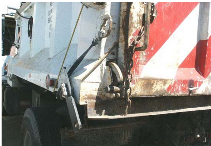
Figure 4-37. Latch on Tailgate of Haul Truck.
