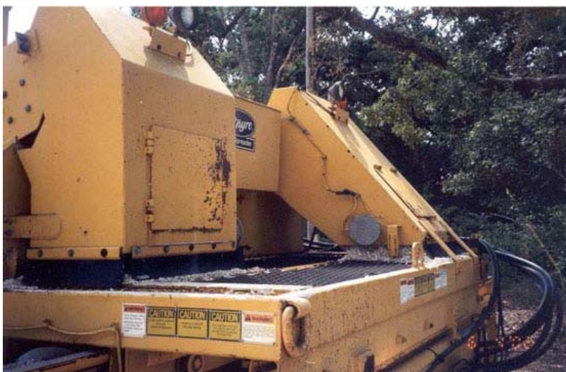
Figure 4-31. Discharge Hopper of Aggregate Spreader.
