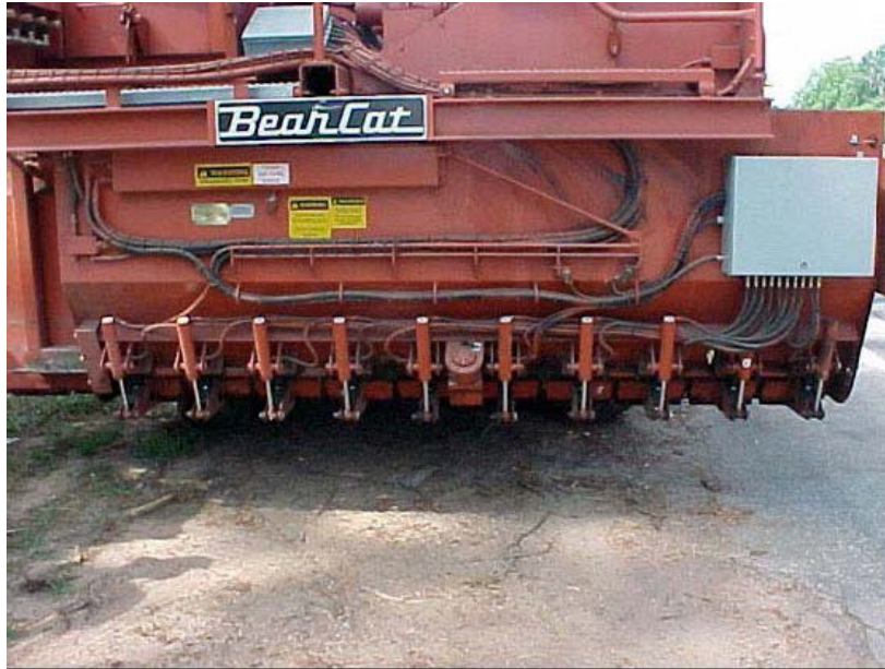
Figure 4-32. Discharge Gates on Aggregate Spreader.
