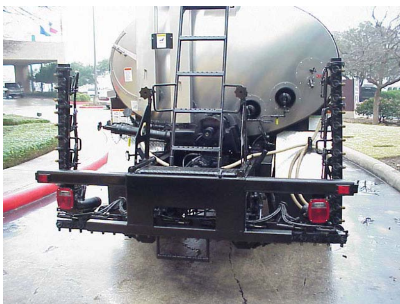
Figure 4-13. Hinged Spray Bar with Ends Folded Up.
