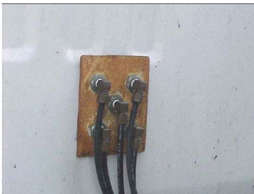
Figure 4-34-A. Air Line Connections on Back of Truck Cab.
