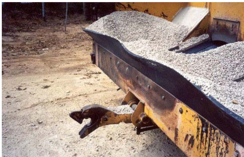
Figure 4-28. Aggregate Spreader Truck Hitch.
