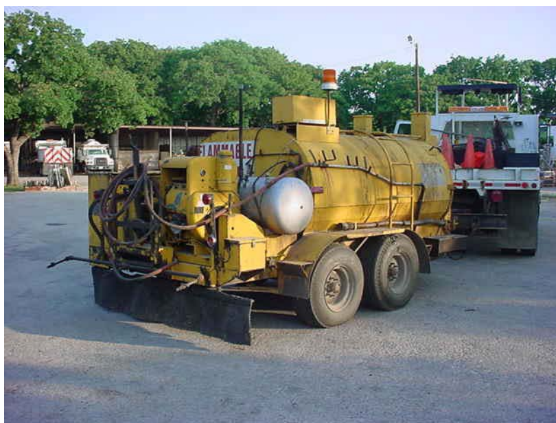
Figure 4-10. Trailer-Mounted Asphalt Distributor.
