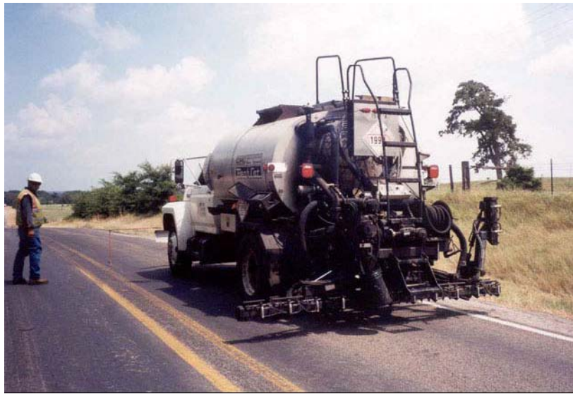
Figure 4-11. Typical Distributor Spray Bar.
