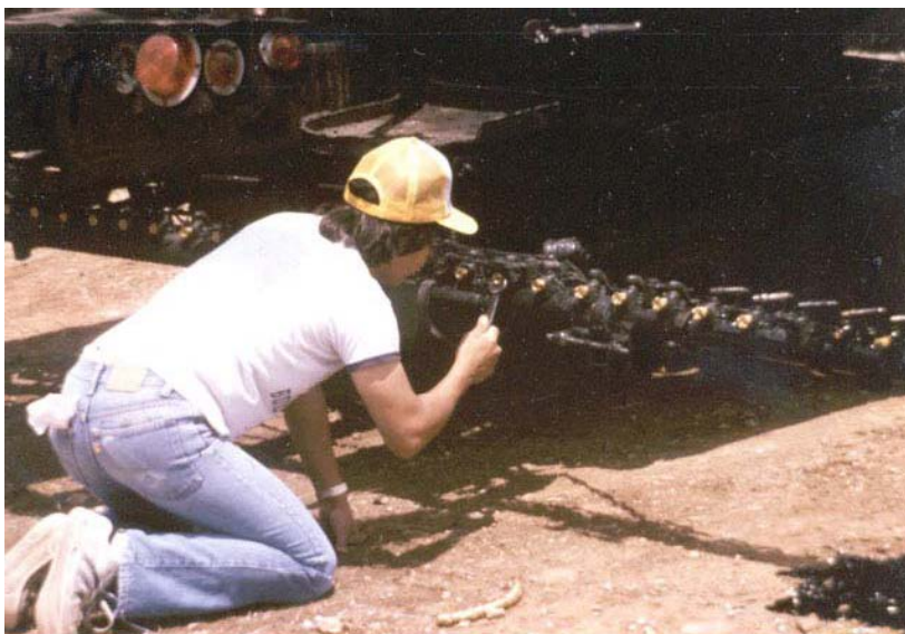
Figure 4-16. Distributor Spray Bar Rotated Outward.
