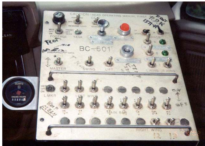
Figure 4-26. Computerized Asphalt Distributor Controls.
