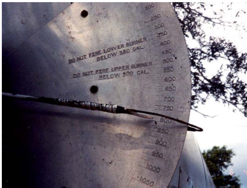
Figure 4-24. Volume Gauge on Distributor Tank.
